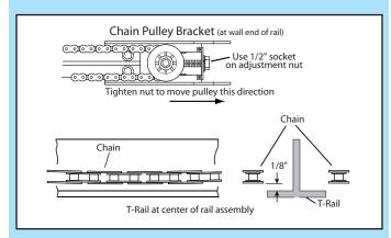
FIG. 1-6 Chain adjustment.
